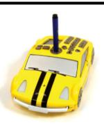
The robot features four built-in sensors which can activate procedures from touch, light and sound.
